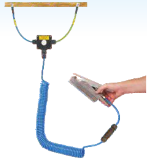
Bond-Rite CLAMP supplied with 2 conductor cable, junction box, clamp stowage pin and grounding leads. Circuit monitoring board and battery mounted inside clamp. Grounding bus-bar not supplied.
